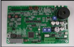
**A-208 Swept Frequency Board.** New revision features better noise handling and built in alarm and frequency counter and can also with an optional IR have people counter built in.
